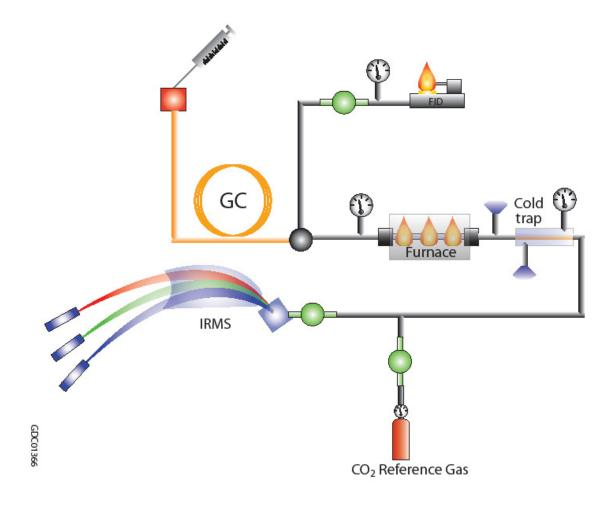
111. In an anti-doping laboratory the GC is coupled to a combustion carbon isotopic ratio mass spectrometry (GC/C/IRMS indicated also by the abbreviation GC-IRMS) to discriminate between the endogenous and the synthetic origin of
