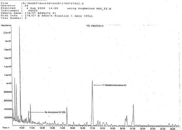
**126.** The peaks of interest according to the first fraction GC/MS run are 5-alpha AC (the chromatographic reference standard) and 11-ketoetiocholanolone.
