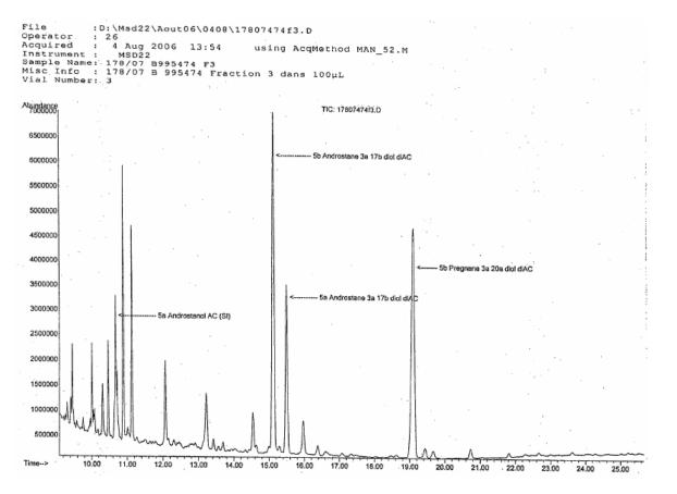
128. The GC/MS run of sample fraction 3 indicates there are 4 peaks of interest representing, 5-alpha AC (the chromatographic reference standard), 5 betaandrostandiol, 5 alpha androstandiol and lastly, 5 beta pregnandiol.
